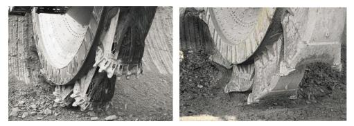
Fig. 7. a) Chain mat instead of shell of buckets b) bucket with corner cutters for soft material
