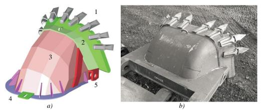
Fig. 6. Typical bucket design 1 Tooth, 2 Lip, 3 shell, 4 attachments a) rounded b) rectangular
