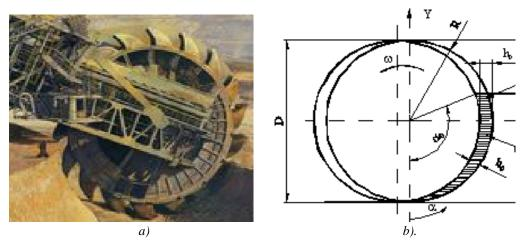
Fig. 5. Typical bucket wheel (a) cutting height relative to BW diameter (b)
